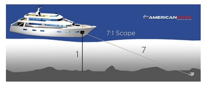
To determine how much rope to let out to get a 7:1 scope, you measure the depth of the water, add the boat's freeboard at the bow, and multiply that sum by 7. But, knowing the length won't help you a bit unless you can determine when you have let out that much rope. So, the very first thing to do with your new anchor line is to mark it. You can do this with a marking pen, but short yarns or tapes inserted throughout the strands is more durable and can be identified in the dark by feel.
